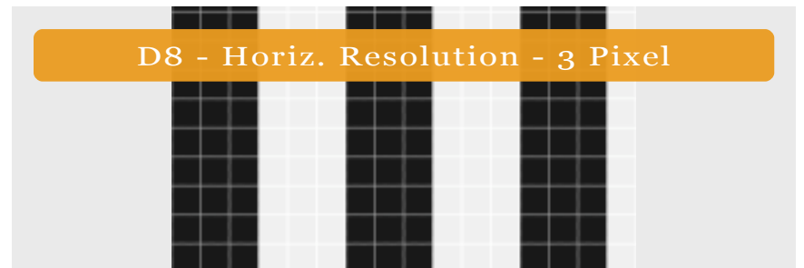
The original unscaled video contains three pixel wide columns that alternate between black and white.
