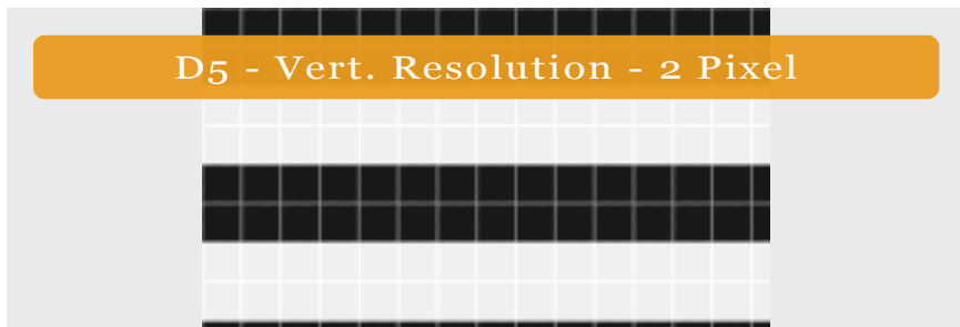
The original unscaled video contains two pixel wide lines that alternate between black and white.
