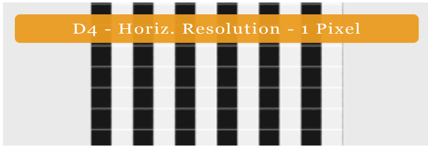
The original unscaled video contains single pixel wide columns that alternate between black and white.
