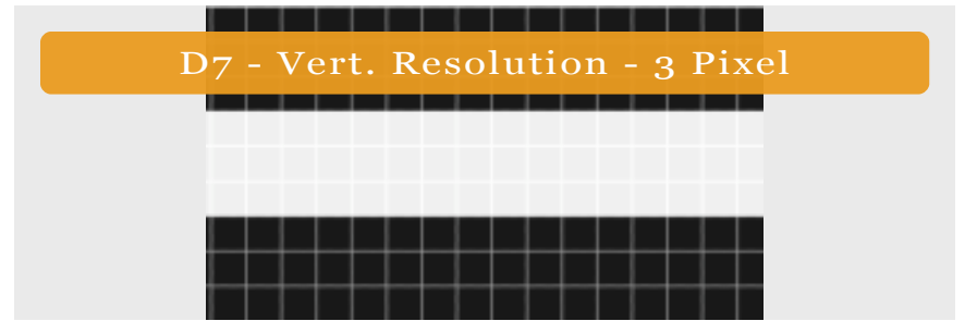
The original unscaled video contains three pixel wide lines that alternate between black and white.
